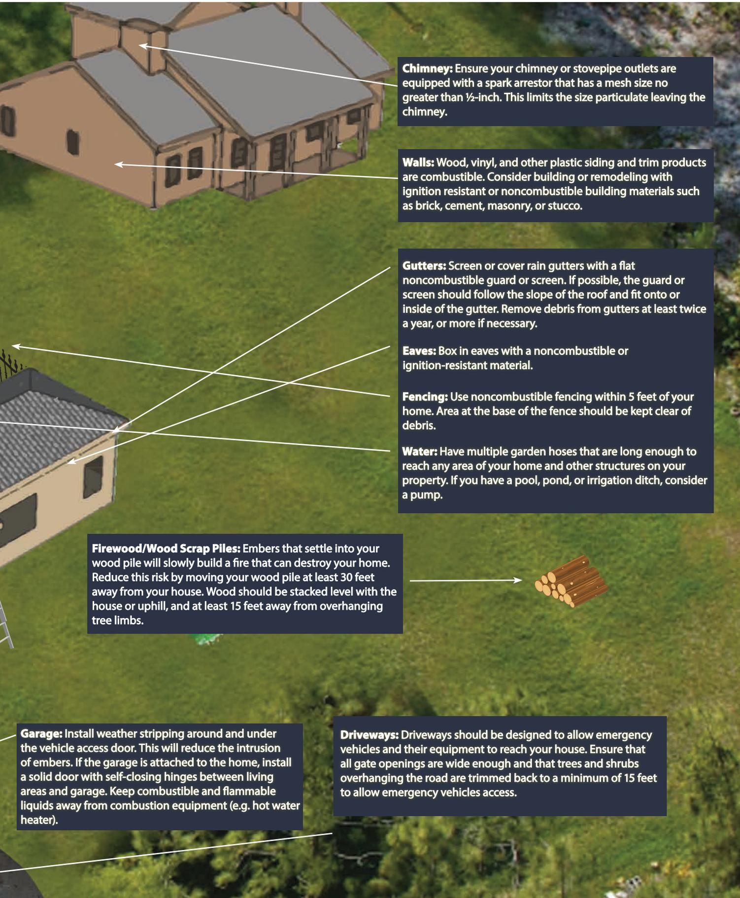
**Chimney:** Ensure your chimney or stovepipe outlets are equipped with a spark arrestor that has a mesh size no greater than ½-inch. This limits the size particulate leaving the chimney.
